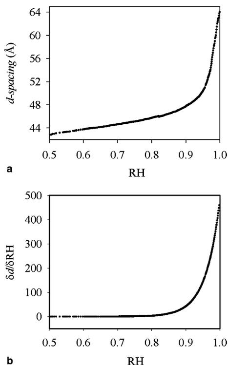
Fig. 4. Evolution of the lamellar  $d$ -spacing as a function of RH (a) and its first derivative,  $d' = \delta d / \delta RH$  (b), that allows to detect two distinct hydration regimes. In the first one ( $0.5 < RH < 0.9$ ),  $d$  linearly increases and the  $d'$  is nearly constant. In the second one ( $RH > 0.9$ ), an abrupt increase of  $d'$  can be observed. This profile shows the extreme sensitivity of  $d$  to RH in the humidity range ( $0.9 < RH < 0.1$ ).
