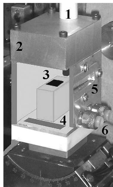
Fig. 2. Photograph of the hydration chamber: humidity controller (1); removable top (2); solid-supported lipid film (3); water reservoir on the bottom of the cell (4); mylar entrance window (5); refrigerator water circulator (6). The hydration chamber is mounted on a rotation motor that allows to align the membranes respect to the incident X-ray beam.
