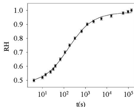
Fig. 3. Temporal evolution of measured RH. Solid line is the best fit to the data obtained applying Eq. (1).
