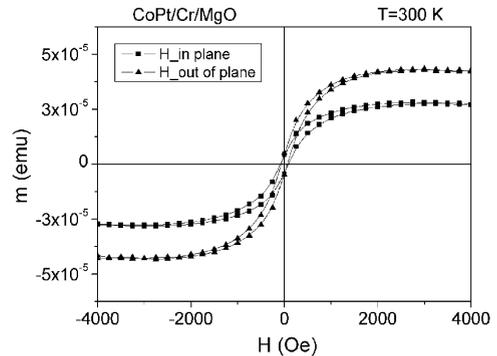
Fig. 3. Hysteresis cycles at room temperature for  $H$  parallel and perpendicular to the film plane.
