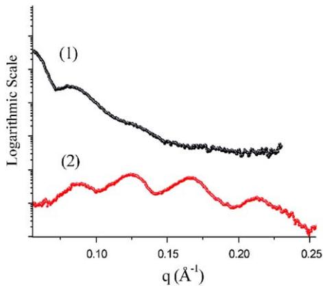
Fig. 2. EDXR experimental data for films deposited at  $500^{\circ}\text{C}$  (1) and  $100^{\circ}\text{C}$  (2): the roughness of the CoPt layer increases with increasing deposition temperature as shown by the faster dumping of the oscillations.
